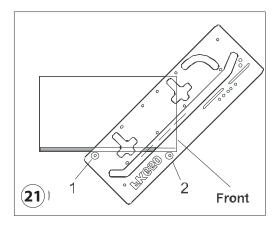
Insert the metal stops into the holes. Fix the jig FK to the edge of the worktop using the stops. Tighten the jig to the kitchen worktop using the clamps and check that the clamps do not hinder the movement of the router. Set the cutting depth on the router. Insert the router and begin to cut the joint on multiple-pass from left to right.
