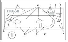
Tighten the jig to the kitchen worktop using the clamps and check that the clamps do not hinder the movement of the router and that the jig is well tightened to the kitchen worktop. Loosen and remove the sliding length stop to prevent its damage. Set the cutting depth on the router. Insert the router and begin to cut the joint on multiple-pass from left to right. Copy the far edge of jig FK (fig. 12).
