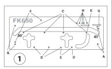
Cutting of inner part of joint using the sliding stop
